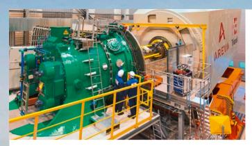
In the full-load test stand, which is equipped with PC-based automation technology from Beckhoff, each Areva M5000 offshore wind turbine is subjected to extensive tests.
