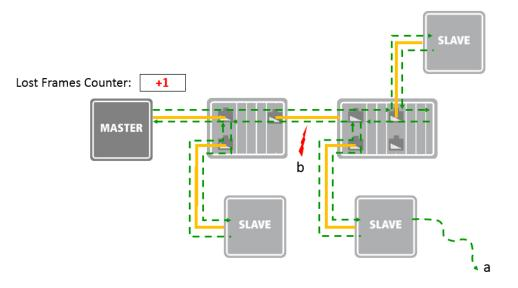
The master Lost Frame Counter can be considered as the first indicator of communication issues at hardware level in an EtherCAT network: an increment should trigger a deeper investigation by reading and interpreting <u>Hardware Error Counters</u> of slave devices.
