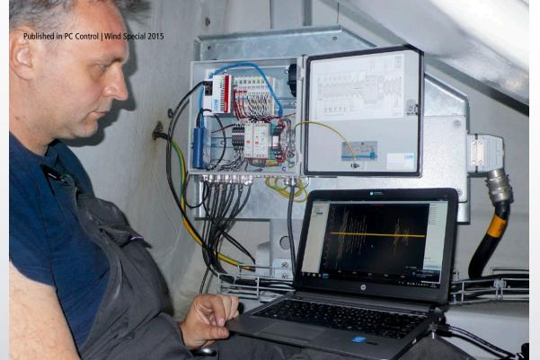
GfM staff engaged in testing acceleration sensors connected to the Peakanalyzer.
