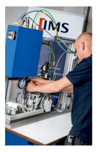
The plug-in production modules can be tested offline and installed according to the plug-and-play principle.
