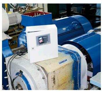
The EMCM developed by Končar is a comprehensive online condition monitoring system for low-voltage and high-voltage induction motors of any size.
