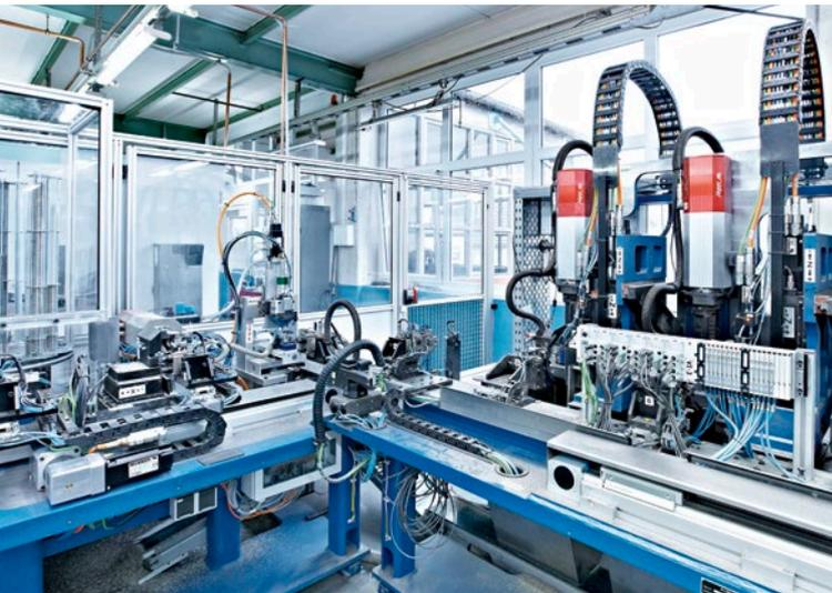
The interlinked key production line designed by Aumat and AST, consisting of a key cutting machine and a profile milling machine, machines key blanks with high precision down to lot size 1.
