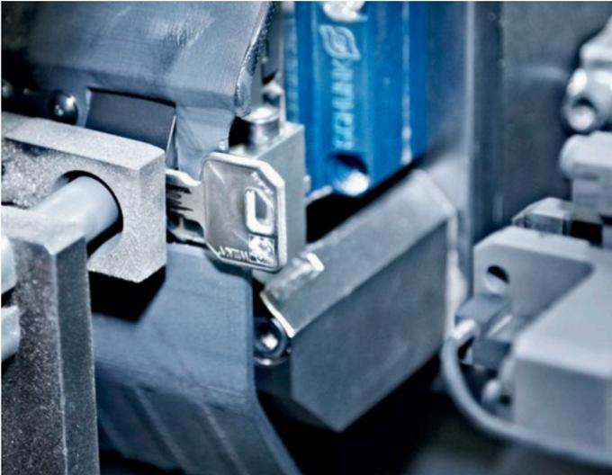
According to the order, the key blanks first receive the desired longitudinal profile and then the notches of the key bit.
