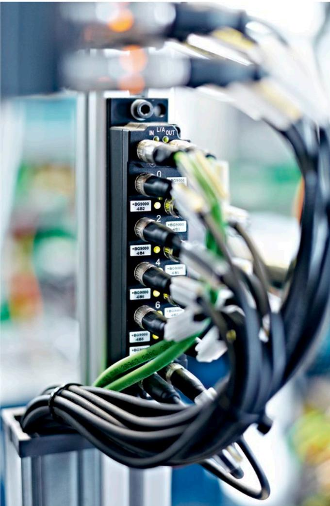
In the process, decentralized collection of I/O data via the EtherCAT Box modules, EP1008 and EP2028, directly on-site reduces the required control cabinet space to a minimum.
