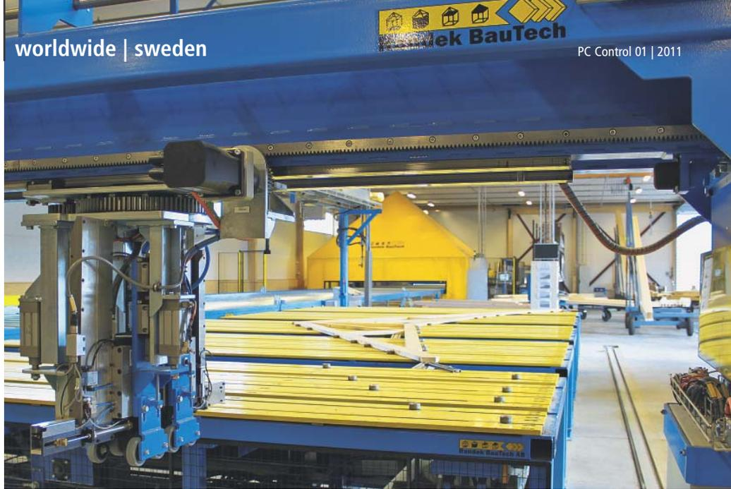
The fully automated production line from Randek represents a big step forward in speed, economy and quality for the manufacture of nailed roof trusses. A new roof truss, the load-bearing component of the roof frame, rolls off the conveyor belt every 81 seconds. The production plant is controlled by a PC- and EtherCAT-based control platform from Beckhoff.
