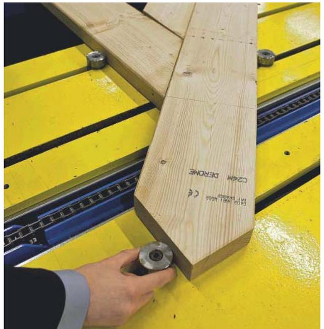
The automatic press visually identifies the butt joints in the roof truss design and positions the nail plate exactly on the joint. It then presses this into the timber with the necessary pressing force and creates a perfect joint. After all the butt joints have been fixed with nail plates, the roof truss is transported to the next station.
