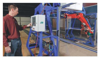
The USBC personnel can easily enter the test settings via a Beckhoff CP6901 Control Panel with a 12-inch touch screen display. There are 11 variables for configuring different throws to adjust speed and pick-up orientation. The E.A.R.L. robot can be reconfigured for completely different parameters in less than 10 seconds.
