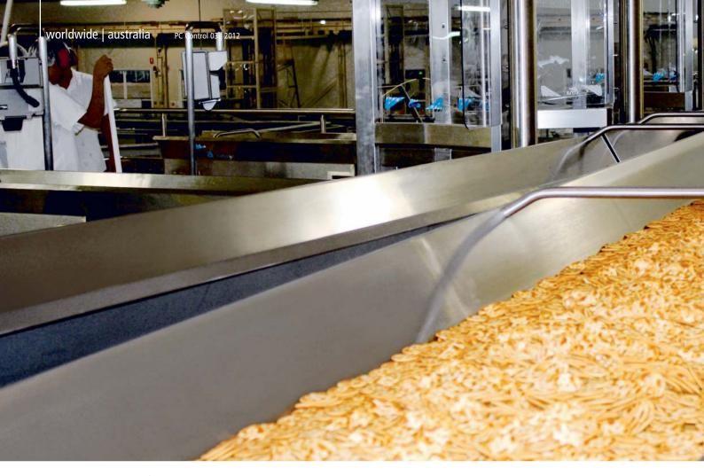
The product is moved carefully in the pans. Once the desired position is reached the pan opens and the product is discharged.
