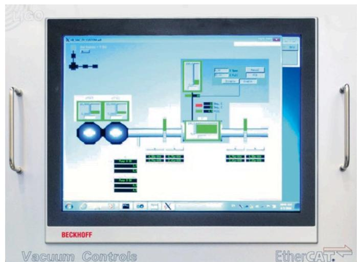
The vacuum control systems developed by LIGO heavily utilize PC-based control and EtherCAT communication technology.
