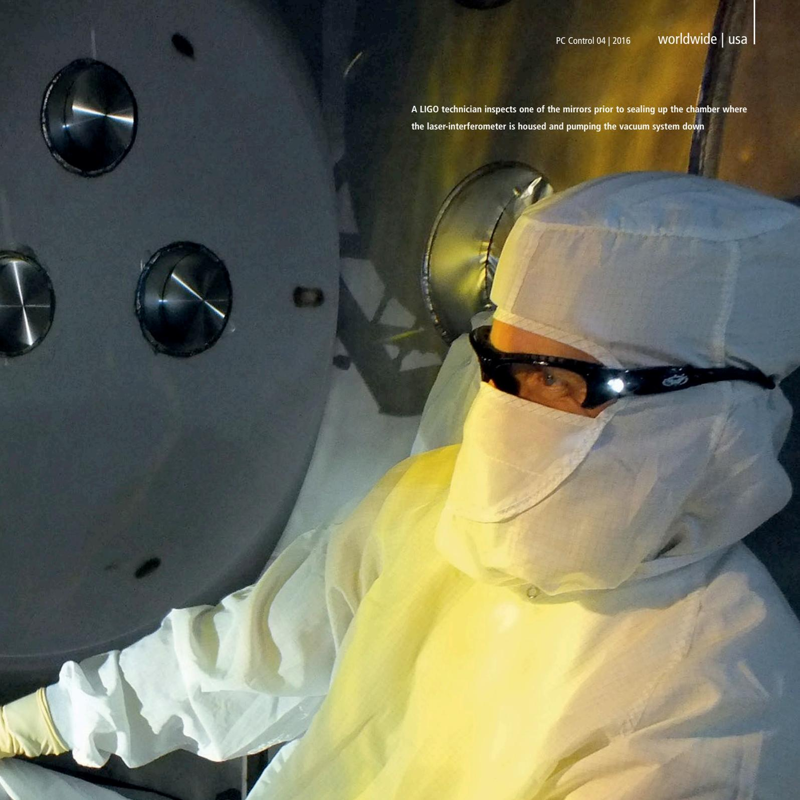
A LIGO technician inspects one of the mirrors prior to sealing up the chamber where the laser-interferometer is housed and pumping the vacuum system down
