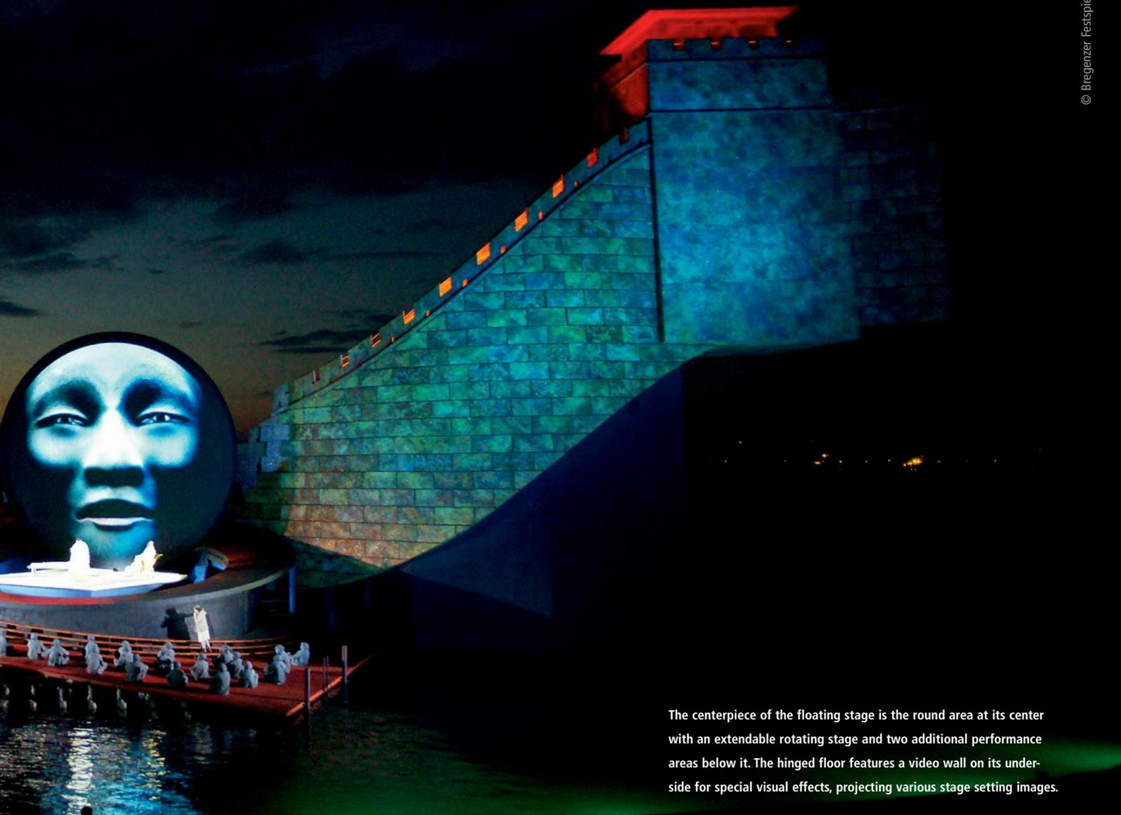
The centerpiece of the floating stage is the round area at its center with an extendable rotating stage and two additional performance areas below it. The hinged floor features a video wall on its underside for special visual effects, projecting various stage setting images.
