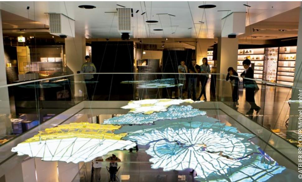
The projection surfaces are suspended on 30 steel cables. Their movement through the three exhibition levels with a height of around 15 meters is individually controlled by servomotors. A total of eight projectors are installed, five of which on the ceiling of the third floor and one each on the other three floors.
