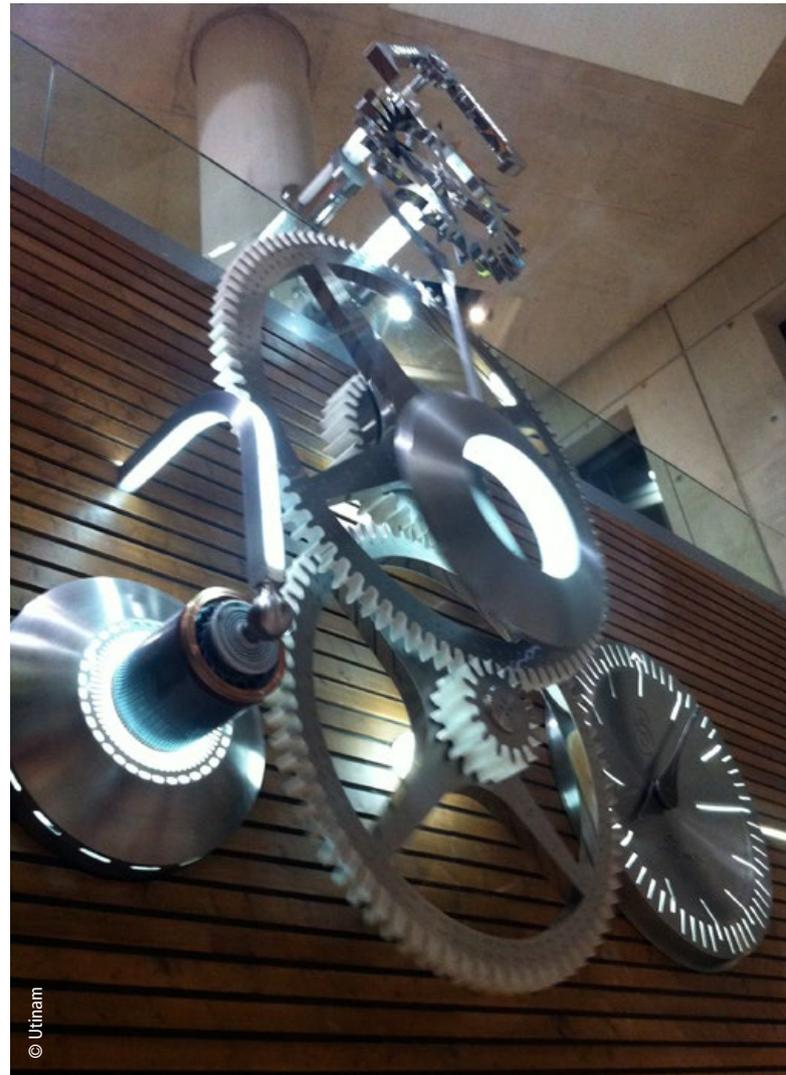
The eye-catching clock which Utinam designed for the TGV station in Besançon has no housing, making its mechanisms fully visible. With its considerable height of six meters, it stretches over two floors. The escape wheel, which links the mechanisms to the pendulum, has a diameter of 1.44 meters while the hour wheel measures 2.85 meters.
