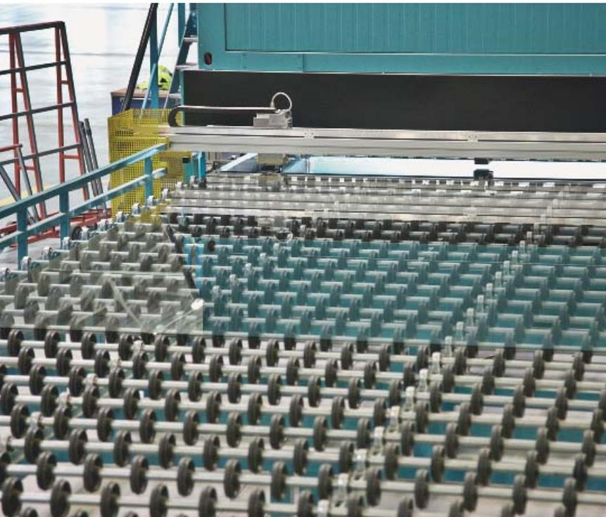
Quality control follows the coating process. Optical sensors measure the light reflection and transmission of the glass panes before the electric resistance is measured.
