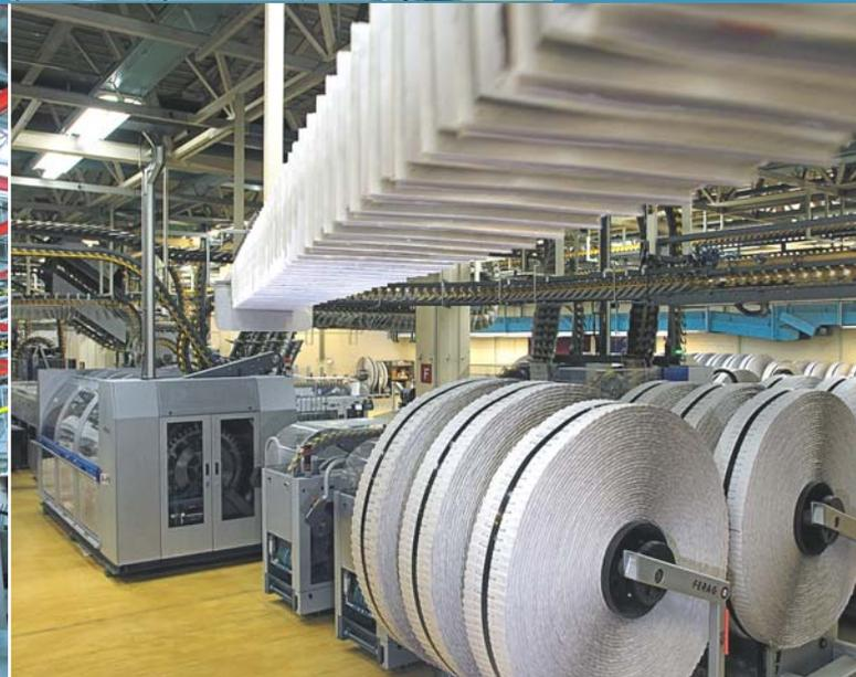
Printing on the fly: for a perfect finish, the positioning of the newspaper and the printing of the address in the field provided on the cover sheet must be synchronized precisely.
