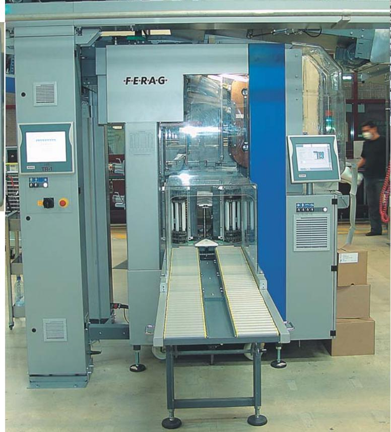
The Beckhoff CP77xx and CP69xx Control Panels are used as operating terminals and were manufactured as custom versions especially for Ferag. The CP62xx Panel PC version is also used.
